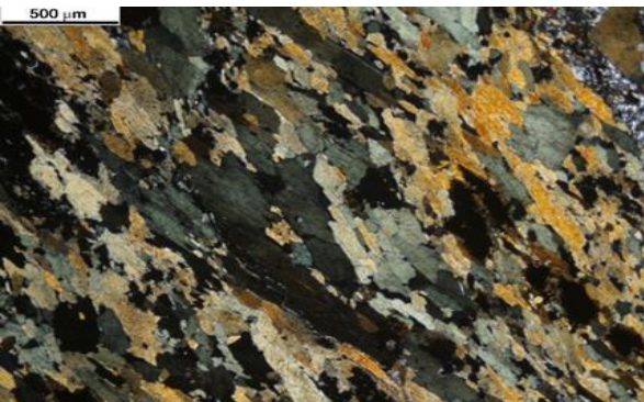
Fig (11) Photomicrograph in the present foliated amphibolite showing well developed foliation represented by amphibole minerals. (X.P.L).
